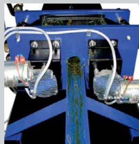
Rotation direction and speed- controlled 24 V DC motor.
